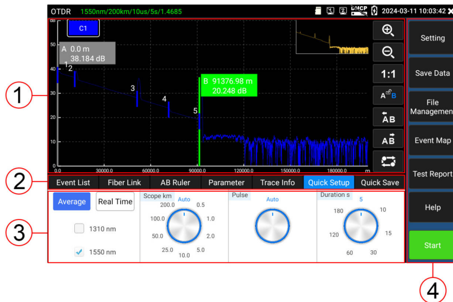
① Trace area ② Trace operation button area ③ Information area ④ Menu button area
